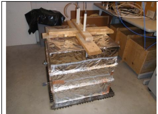
Figure 2. Soil filled box insulated with grounded tin foil
