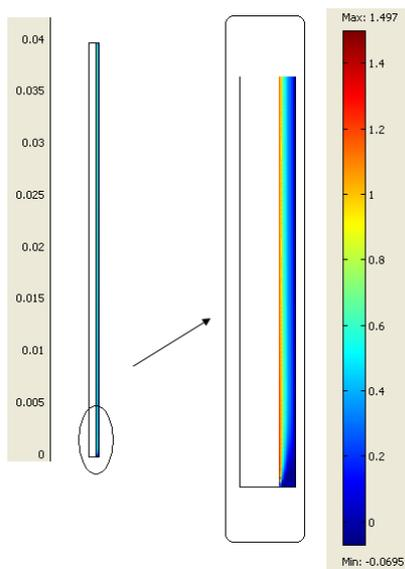
**Figure 5.** Velocity profile in the porous layer
