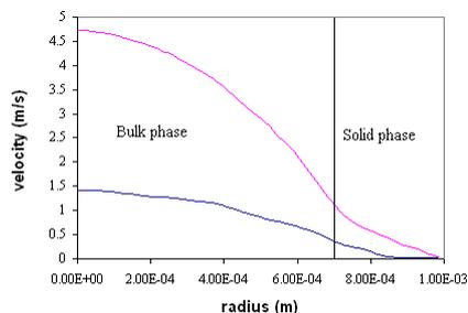
**Figure 8.** Velocity profile for cases 1 (up) and 4 (down)
