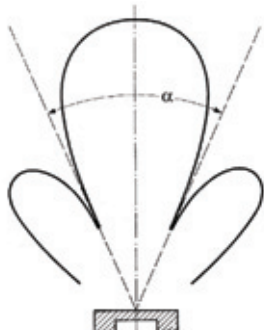
Figure 4: Directivity (logarithmic diagram) of a plane piston in the far field [1]
